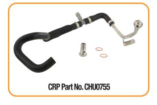
equipped with the twin turbocharged V8 4.4L engines (CRP Part No. CHU0755). The OE version of this hose features a plastic T-fitting, which is known to fail. The upgraded Rein version of this coolant line includes a **metal T-fitting** that eliminates the common failure point to ensure a longer, problem-free life.
