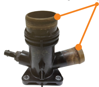
Example of Plastic Connector Damage from Hydrolysis
